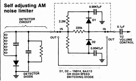
This is a very effective self-adjusting positive and negative peak noise limiter. The detector diode is part of the usual detector arrangement in a receiver and provides a negative bias which varies with the average signal strength (bias provided by D1 and D2). When a noise spike appears on the positive swing of the demodulated audio wave form. D1 conducts flattening out the spike. Similarly when a noise spike appears on negative swing of the audio, D2 conducts flattening out the spike.
